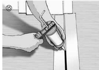
In doorways you should mount a suitable moulding system to cover the expansion gap. This also applies if the same floor is to be laid in the adjoining room. A 5 mm (0.2 ") expansion gap, closed with a matching colour acrylic, must be provided. With work on tile surfaces and fixed components that are not covered with skirting, from a length of 150 cm (5 ft.) the expansion joint is no longer to be closed with acrylic, but rather must be covered with a suitable moulding system.
