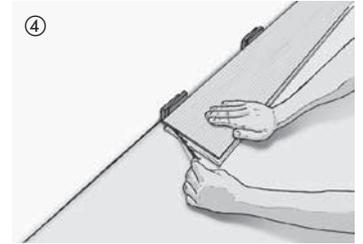
The boards of the first two rows are laid alternating **without removing the protective film at first**; when the surface is finished the first two rows are removed again and the protective film is removed. To remove it later on the plastic tongues must be removed from the short sides and kept stored.
