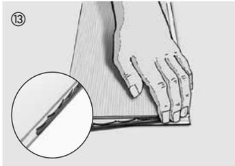
The removed tongue (see point 4) must first be inserted back into the short side joint. Please pay attention to the plastic bevel that faces up when replacing the tongue. The "split end" (see picture detail) will point to the long side of the groove if the tongue is positioned correctly.
