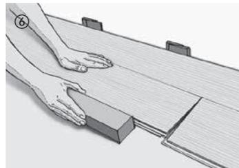
To lay the next boards of the second row (**also with the protective film**) the board is angled into the previous row along the long side by applying a small amount of force into the joint (groove). The long side is also tapped in lightly with the tapping block if required.
