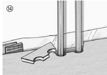
If radiator pipes protrude from the floor, drill or saw a cutout into the board, leaving the required expansion space. As a rule, a fine saw must be used to cut a gap the thickness of a board in wooden door frames to allow the laminate floor to expand.
