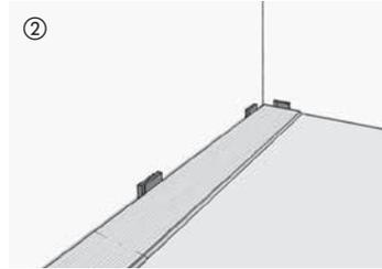
Start installation in the right corner of the room. Lay the first board and fix it to the wall with distance spacers **without removing the protective film**. The expansion gap to the wall should be 10–15 mm (0.4"–0.6"). Always align the boards with the tongue side parallel to the wall.
