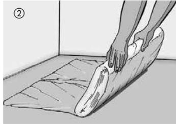
Always use 0.2 mm thick PE film overlapped by 30 cm as an underlay when laying your floor over floor screed. This should overlap in the 30 cm impact area. Extend underlay up all walls. After having installed the skirtings cut underlay at the upper edge of the skirtings. **As the HARO cork floor already has an integrated cork insulation layer, do not use any additional insulation underlay.**
