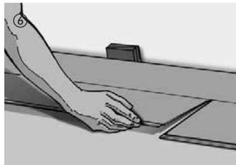
The next row is started with the leftover piece of the first row (short side offset of at least 40 cm). This considerably reduces waste. The rest of the installation is performed board-by-board. First, the boards are angled into the previous row along the long side by applying a small amount of force.
